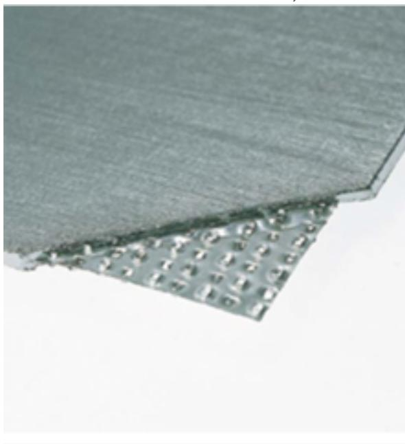
The purity of graphite used is 98% with tanged stainless steel insert AISI 316
